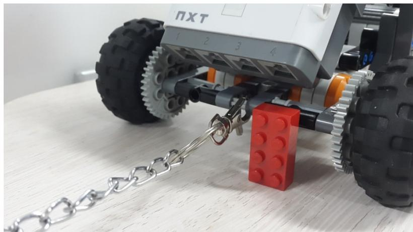
7. The position of the connecting axle must not be further inside the robot's body compared to the outer most part of the robot which is touching the ground (ex: wheel). As an example, look at the illustration below:
