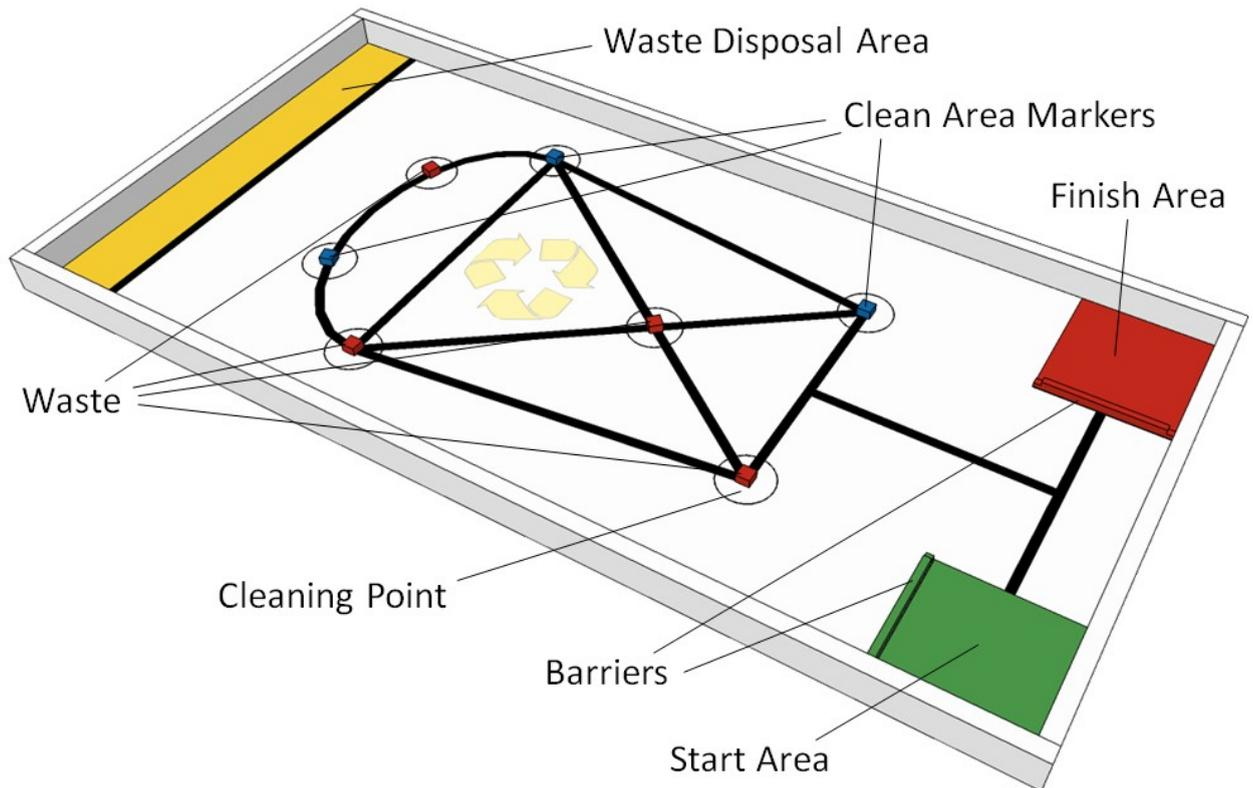
The robot will start from within the start area (green square) carrying 4 blue LEGO blocks to be used as "clean area markers". Randomly placed in the 7 circles are 4 red blocks and 3 blue blocks.
